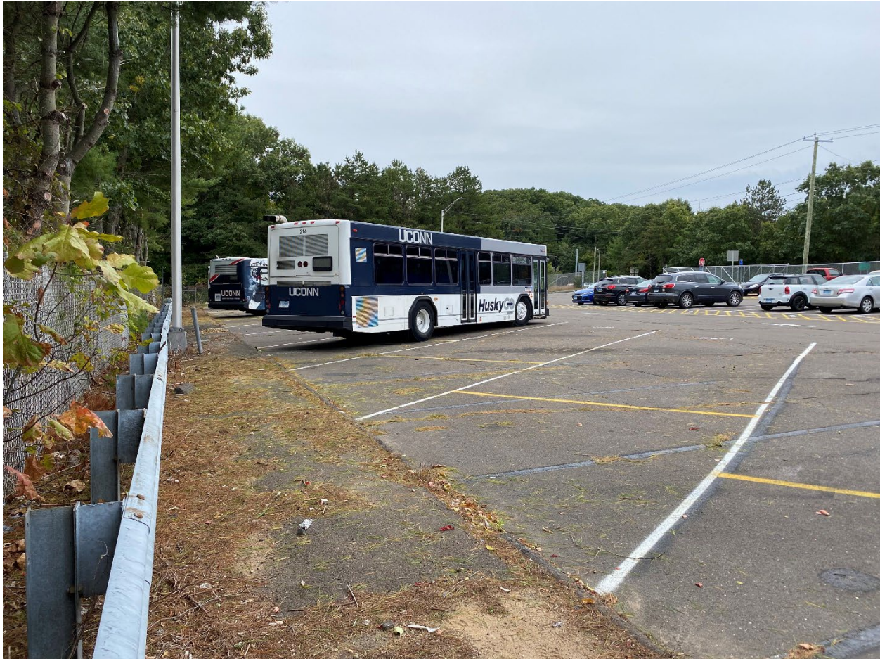
Figure 2 The buses back into the spaces and will need to be connected from the back of the bus. The conduit would be mounted on the back side of the beam rail in lieu of underground trenching. A duplex receptacle will be placed in between two buses.
