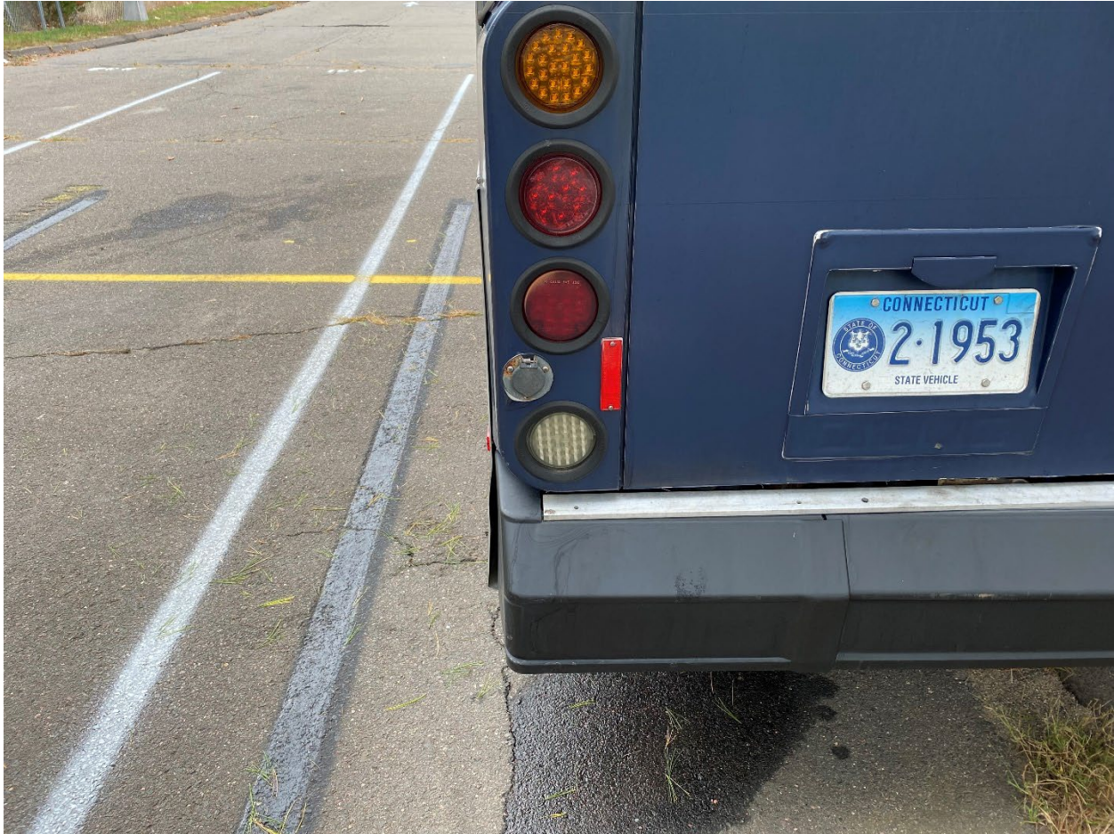
Figure 6 The connection to each bus is made from the back of the bus. The bus provides the male straight blade connection that mates with the outlet or female end of an extension cord.
